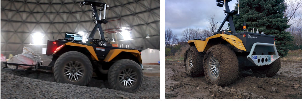
(a) The Grizzly loaded with gravel bags in the UTIAS Mars Dome. Data from this configuration was used to compare the predictive performance of GPs and wBLR in Sec. 4.6. (b) The Grizzly on the muddy test track used for the closed-loop comparison between GPs and wBLR in Sec. 4.7.
