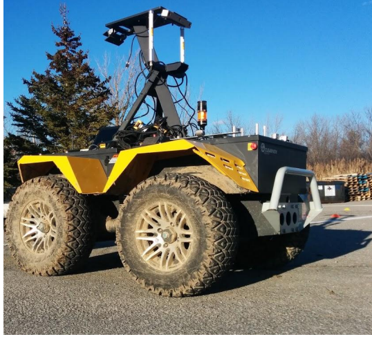
Figure 5.3: The Clearpath Grizzly with mast-mounted stereo camera used for the experiments in this paper.
