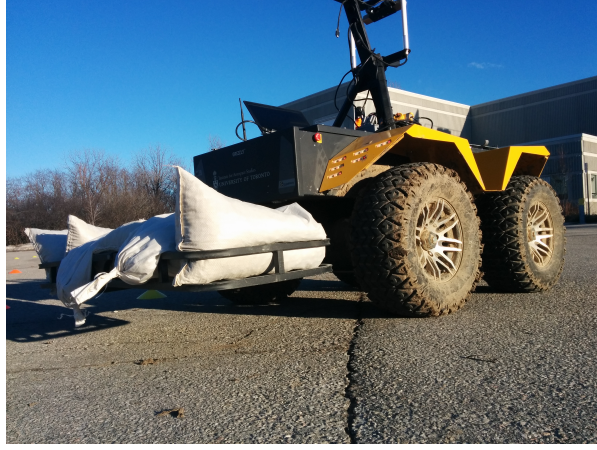
Figure 3.9: Clearpath Grizzly in the loaded configuration with six bags of gravel in the cargo carrier. Each bag weighs approximately 30 kg for a total payload of 180 kg.
