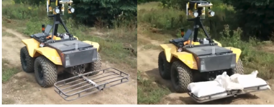
Figure 6.2: The Clearpath Grizzly in nominal (left) and loaded configurations (right). The mass of the bags of gravel was 133 kg.
