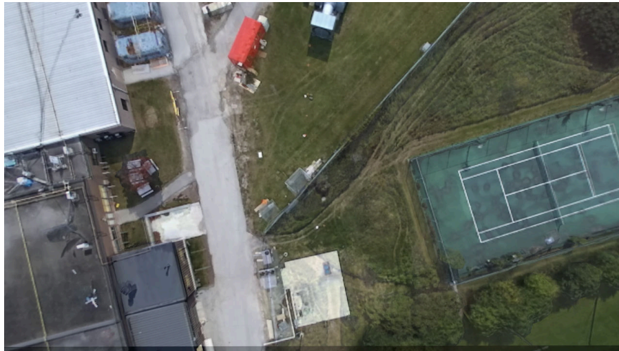
(c) Alpha blended image of the UAV query image (prominent) and the Google Earth map image warped with the optimal sRt parameters from the refined optimization.
