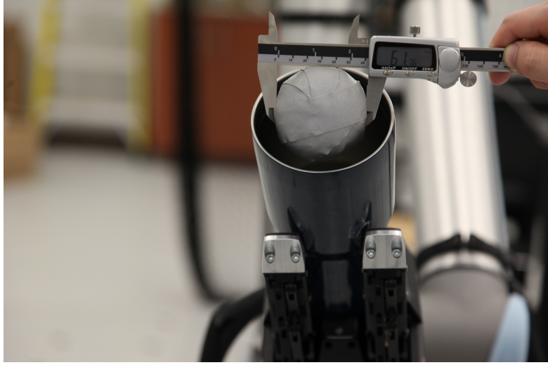
Figure 3.7: The 61.76 mm diameter ball and 94.90 mm diameter cup used in this paper. The position accuracy requirement in the x, y, z axes is approximately (94.90 - 61.76)/2 = 16.57 mm. The typical speed at the catch time is around 5 m/s, leading to the 16.57/5 \approx 3 ms time precision requirement.
