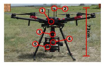
Fig. 1. The experimental setup for VT&R on our multirotor UAV: (1) DJI Matrice 600 Pro vehicle platform, (2) DJI A3 triple-redundant GPS module, (3) DJI Ronin-MX 3-axis gimbal, (4) NVIDIA Tegra TX2, (5) StereoLabs ZED camera.
