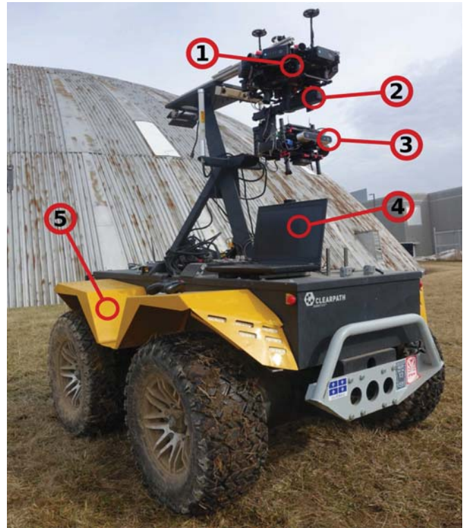
Fig. 1: The experimental setup for gimbal-stabilised VT&R: (1) DJI Matrice 600 multirotor body, (2) DJI Ronin-MX 3-axis gimbal, (3) StereoLabs Zed stereo camera, (4) Lenovo W541 Intel Core-i7 laptop, (5) Clearpath Grizzly RUV.
