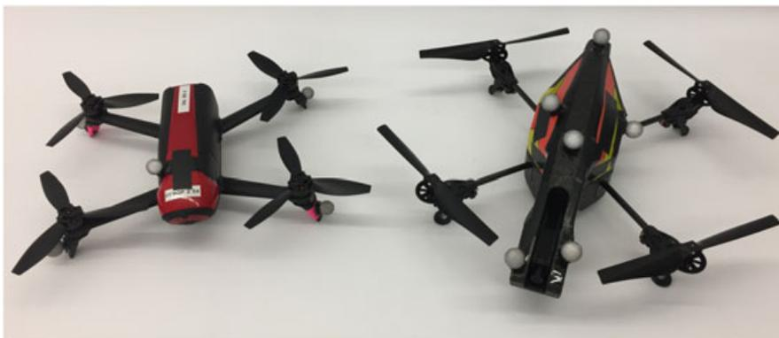
**FIGURE 3** Vehicles used in the experiments. On the left the Bebop 2, on the right the AR.Drone 2.0 [Colour figure can be viewed at [wileyonlinelibrary.com](http://wileyonlinelibrary.com)]
