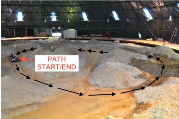
Fig. 8. Experiment 2: ROC6 at the start of the path in the MarsDome facility in Toronto, Ontario, Canada. The facility provides a network of sandy and gravel floor valleys defined by a set of impassable gravel hills. A supplemental video presenting this experiment is also available at <http://ieeexplore.ieee.org>.
