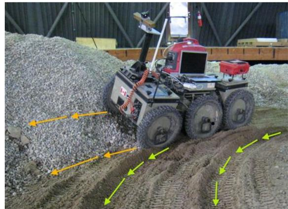
Fig. 2. ROC6 robot tracking a path at three times the nominal safe speed of 0.35 m/s. The orange arrows show the current trajectory of the robot as it drives with ILC disabled. The green arrows show the path with reduced errors from when the robot learned to travel at speed with ILC enabled.
