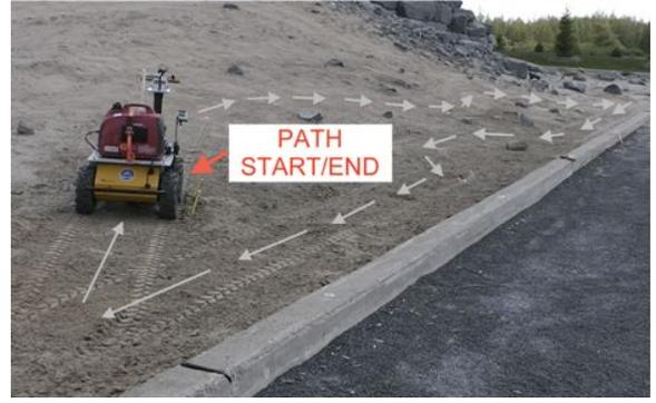
Fig. 6. Experiment 1: Husky A200 path at the Canadian Space Agency's Mars Emulation Terrain in Longueuil, Québec, Canada. The terrain offers a large selection of surface topographies intended for robot mobility testing.
