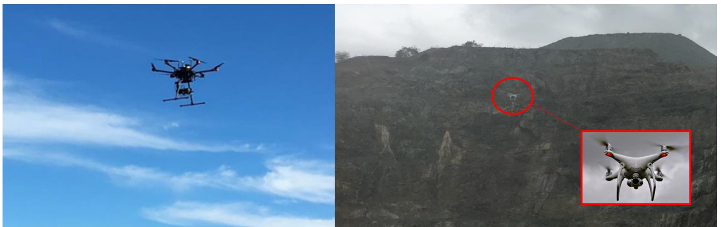
Fig. 2 DJI Matrice 600 Pro with LiDAR setup (left) and DJI Phantom 4 Pro (right).
