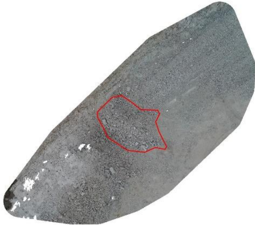
Fig. 9. Orthophoto produced by OpenDroneMap using a set of images captured by the UAV of the muckpile in the Lupita pit. The boundary of the muckpile is represented by the red polygon.
