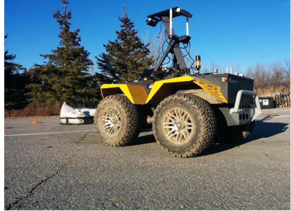
Fig. 3. The Clearpath Grizzly with mast-mounted stereo camera used for the experiments in this paper.
