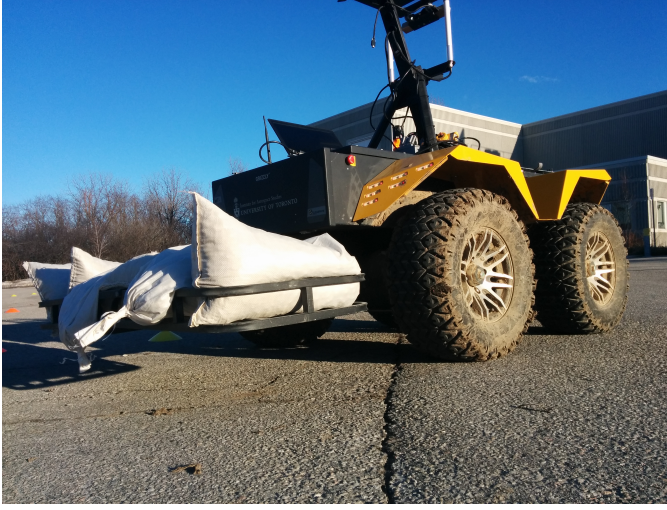
Fig. 3: Clearpath Grizzly in the loaded configuration with six bags of gravel in the cargo carrier. Each bag weighs approximately 30 kg for a total payload of 180 kg.
