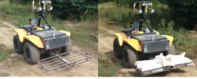
Fig. 2: The Clearpath Grizzly in nominal (left) and loaded configurations (right). The mass of the bags of gravel was 133 kg.
