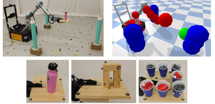
Figure 8: Top left : Real experimental setup. Robot is shown holding the Bottle object. Obstacle locations marked with pylons. Top right : Corresponding simulated experimental setup with collision spheres on the robot in red and on the obstacles in blue. Bottom row : Bottle, Arch, and Cups object arrangements used for experiments. The arch is an example of non-coplanar contact (the three blocks composing the arch are not attached together). The bottle is filled with sugar and the cups each contain bean bags instead of liquid to avoid spills in the lab.
