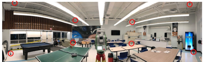
Fig. 9: A panoramic view of the UTIAS cafeteria with the positions of the UWB anchors highlighted in red circles. The dimensions of the cafeteria are 10 m \times 10 m \times 5 m.
