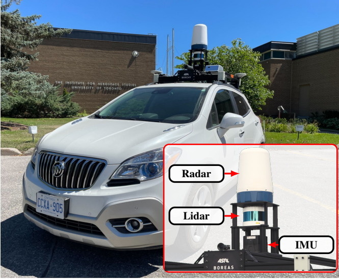
Fig. 14. This figure depicts our data collection platform Boreas which includes a Velodyne Alpha-Prime 128-beam lidar, a Navtech CIR304-H radar, an Applanix GNSS/IMU, and a FLIR Blackfly S camera.
