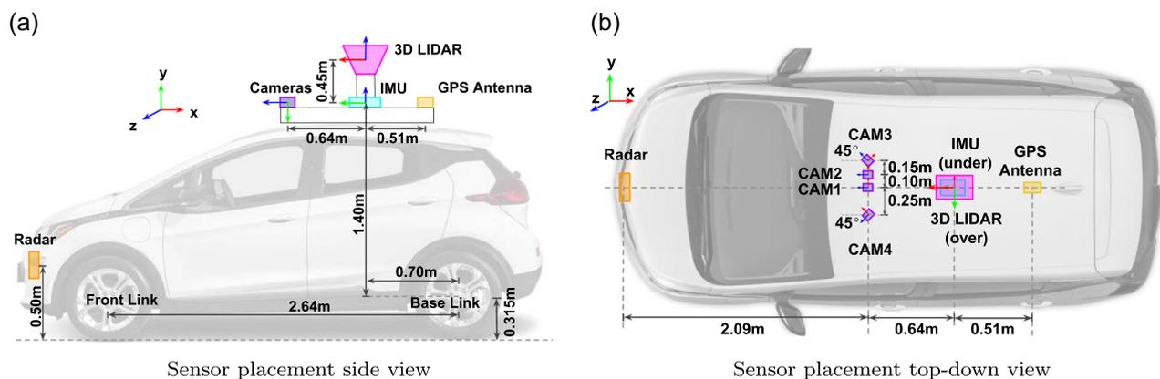
**FIGURE 5** Several sensors are placed along the longitudinal axis of the vehicle. Most sensors are placed so that rotation angles are multiples of 90 degrees. These two factors simplify calibration [Color figure can be viewed at [wileyonlinelibrary.com](http://wileyonlinelibrary.com)]
