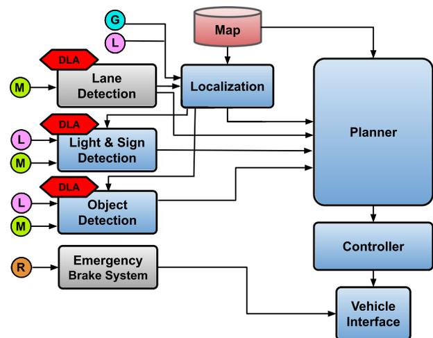
**FIGURE 7** This figure depicts Zeus' software architecture. Localization is either Novatel GPS/IMU or Applanix LIDAR localization. Lane Detection and Emergency Braking (Gray) were not used at the Year 2 competition. DLA, deep learning acceleration; L, 3D LIDAR; M, monocular cameras; R, radar; G, GPS/IMU [Color figure can be viewed at [wileyonlinelibrary.com](http://wileyonlinelibrary.com)]
