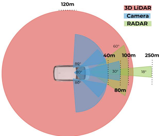
**FIGURE 6** This figure depicts the fields of view of sensors on Zeus. Note that the front-facing cameras provide close to 170 degrees of horizontal field of view. A narrow-field-of-view camera boosts visual detection range [Color figure can be viewed at [wileyonlinelibrary.com](http://wileyonlinelibrary.com)]
