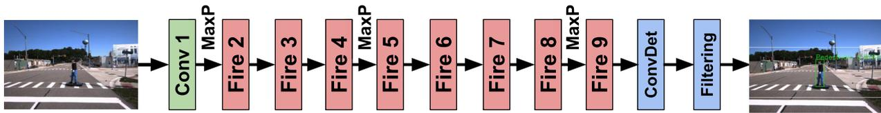
**FIGURE 8** The SqueezeDet architecture. Fire:  $1 \times 1$  convolutions followed by a RELU operation,  $1 \times 1$  convolutions and  $3 \times 3$  convolutions computed in parallel, and another RELU operation. ConvDet: bounding boxes are directly regressed from a dense anchor grid. Filtering, nonmaximum suppression; MaxP, max pooling [Color figure can be viewed at [wileyonlinelibrary.com](http://wileyonlinelibrary.com)]
