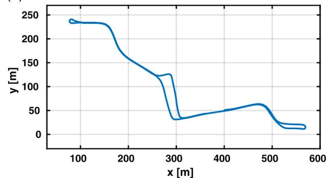
Trajectory output by LIDAR localization
