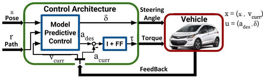
**FIGURE 22** Control architecture for Zeus.  $x$ : current vehicle state;  $u$ : control input [Color figure can be viewed at [wileyonlinelibrary.com](http://wileyonlinelibrary.com)]
