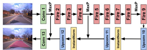
**FIGURE 15** Our proposed semantic segmentation architecture [Color figure can be viewed at [wileyonlinelibrary.com](http://wileyonlinelibrary.com)]
