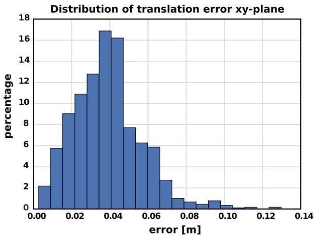
**FIGURE 18** Position error histogram (xy plane) of LIDAR-only localization along a trajectory (see Figure 17) compared to ground truth obtained from postprocessed Applanix POSLV GPS/IMU output [Color figure can be viewed at [wileyonlinelibrary.com](#)]
