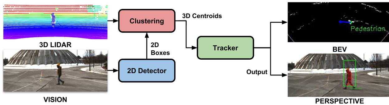
**FIGURE 11** aUToTrack: our pipeline for three-dimensional object detection and tracking [Color figure can be viewed at [wileyonlinelibrary.com](http://wileyonlinelibrary.com)]
