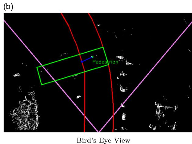
**FIGURE 26** This figure depicts a pedestrian detection from both the perspective and bird's eye view [Color figure can be viewed at [wileyonlinelibrary.com](http://wileyonlinelibrary.com)]
