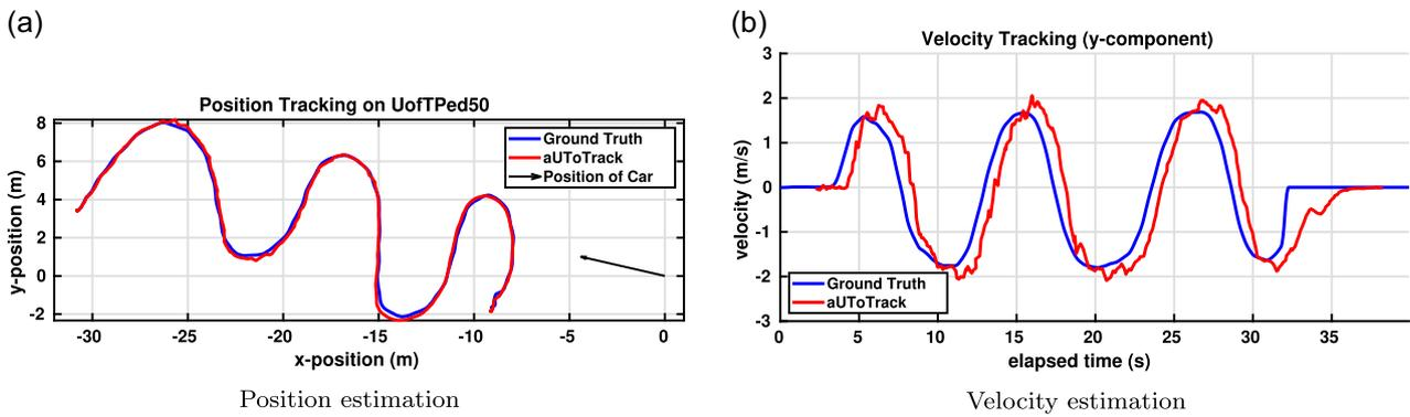
**FIGURE 12** Position and velocity estimation of the Zig-Zag scenario [Color figure can be viewed at [wileyonlinelibrary.com](http://wileyonlinelibrary.com)]
