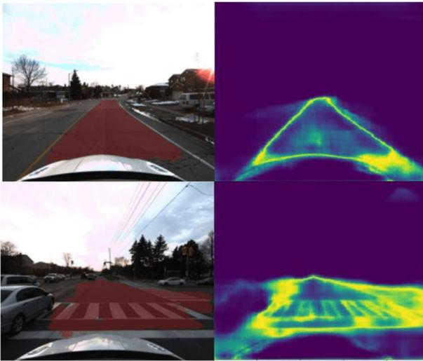
**FIGURE 16** Top: the driving lane is clearly visible. The associated entropy is low. Bottom: the vehicle approaches an intersection. The entropy is high, indicating the lane detection output should be ignored [Color figure can be viewed at [wileyonlinelibrary.com](http://wileyonlinelibrary.com)]
