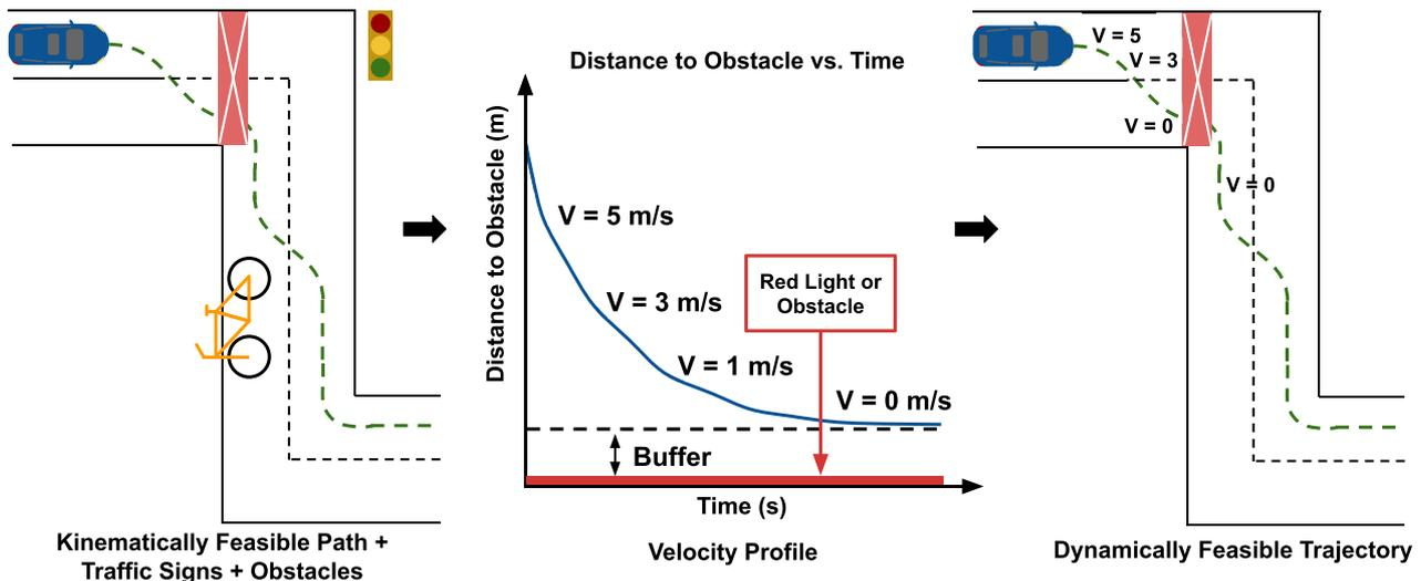
**FIGURE 21** The Velocity Planner uses control points to manage velocity profile along the path [Color figure can be viewed at [wileyonlinelibrary.com](http://wileyonlinelibrary.com)]
