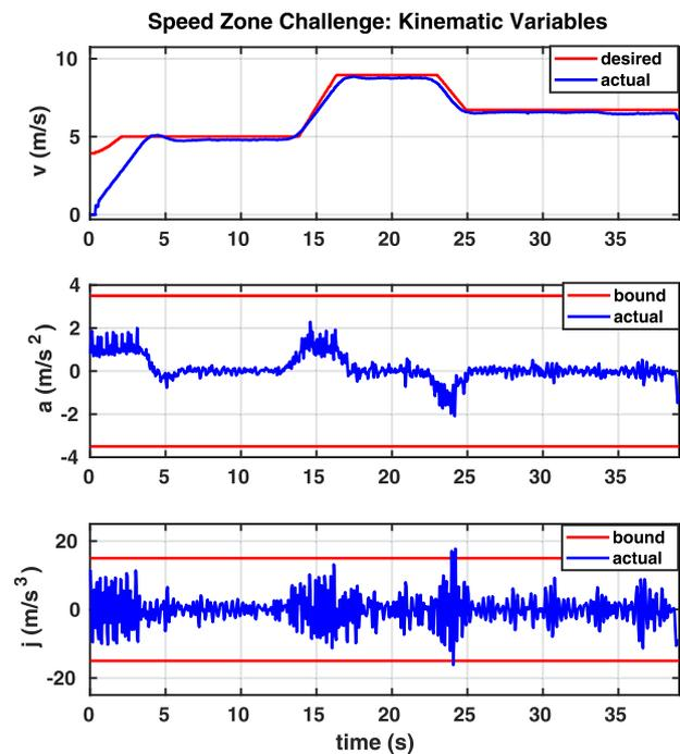
**FIGURE 23** This figure depicts Zeus' performance during the Speed Zone Challenge. The top figure shows the desired velocity alongside the actual velocity of the vehicle. The middle and bottom figures show that we stayed within our acceleration and jerk constraints for the entire course. This data were extracted from Zeus' own sensors during this challenge [Color figure can be viewed at [wileyonlinelibrary.com](http://wileyonlinelibrary.com)]
