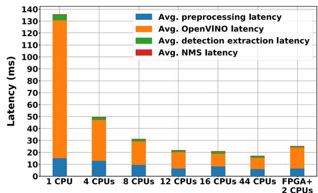
**FIGURE 9** SqueezeDet inference on  $2 \times$  Intel Xeon E5-2699 v4 processors with support of Intel OpenVINO. This figure demonstrates the diminishing returns of accelerating SqueezeDet with CPUs. CPU, central processing unit; FPGA, field-programmable gate array [Color figure can be viewed at [wileyonlinelibrary.com](http://wileyonlinelibrary.com)]
