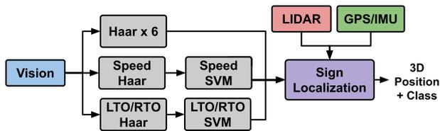
**FIGURE 13** This figure depicts our traffic sign detection pipeline. A generic Haar cascade detector is used to identify speed limit signs and left-turn-only vs. right-turn-only signs. These detections are then classified by a support vector machine for each set. The other six sign classes are detected and classified by a single Haar cascade for each sign [Color figure can be viewed at [wileyonlinelibrary.com](http://wileyonlinelibrary.com)]
