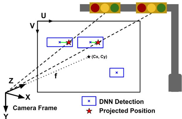
**FIGURE 14** In this figure there are two upcoming traffic lights. Using our position in the semantic map, the locations of these traffic lights are projected onto the image plane (denoted as the red stars). The DNN has output two true-positive detections and one false-positive in this frame (denoted as blue boxes). The green lines denote the association between detections and expected positions [Color figure can be viewed at [wileyonlinelibrary.com](http://wileyonlinelibrary.com)]
