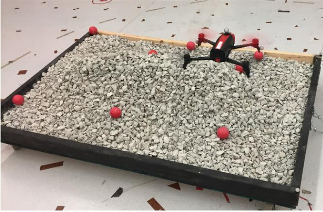
Fig. 2. Aerial vehicle in lab environment conducting aerial fragmentation analysis with known, red scale objects to determine image scale from single 2D images.
