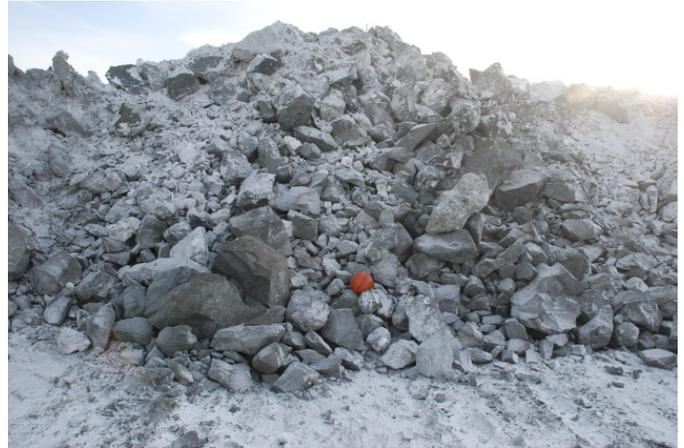
Fig. 1. Typical photo captured during manual image-based rock fragmentation analysis. The scale object (basket ball) is required in order to determine the size of the rock fragments from single 2D images [1].
