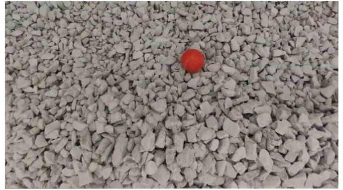
Fig. 6. Raw photo captured in automated aerial fragmentation analysis with scale object to determine image scale.
