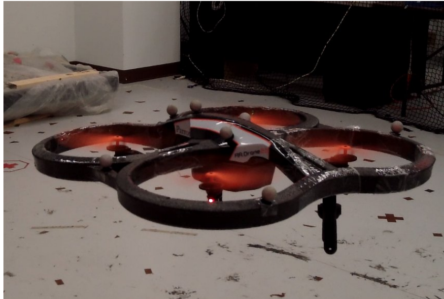
Figure 7.2: Parrot AR.Drone 2.0 showing extruded polypropylene hull and spherical Vicon reflective markers. A clamp is also shown attached to the aft-right landing leg to simulate a mass disturbance.
