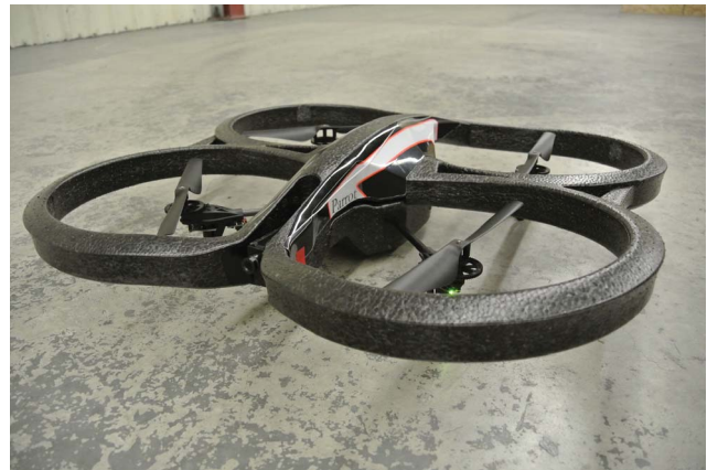
Figure 1. Experiments are conducted at the University of Toronto Institute for Aerospace Studies (UTIAS) using the Parrot AR.Drone 2.0 platform, which is equipped with a downward-facing, monocular camera and altitude sensors. The picture also shows the texture of the floor of the VT&R experiments around the quadcopter.
