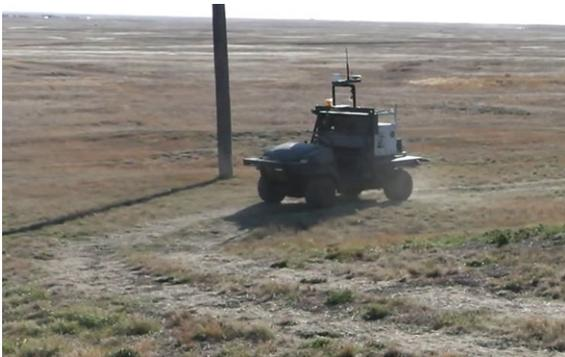
**Figure 16.** In experiment 3, we tested with a 600 kg, Ackermann-steered robot repeating a 100-m-long path. As in the previous experiments, the nominal model used by the LB-NMPC algorithm was a unicycle model, demonstrating the algorithm's ability to be applied to robots with significantly different designs.
