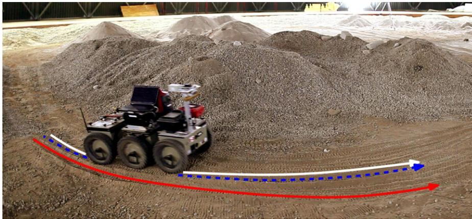
**Figure 11.** The second and third experiments focused on the algorithm’s ability to learn unmodeled robot dynamics. Here we show the skid-steered ROC6 robot driving at 0.6 m/s with learning enabled. The white line shows the desired trajectory (tire tracks), the red line shows a trajectory with learning disabled, while the dashed blue line shows a trajectory with learning enabled and reduced path-tracking errors.
