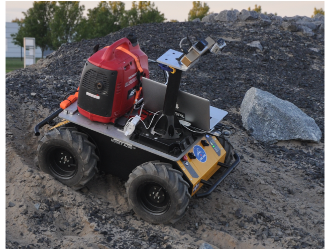
Fig. 1. A Clearpath Husky robot autonomously negotiating challenging terrain with side slopes, inclines, and variable wheel traction. In practice, simple vehicle models rarely represent reality and limit the performance and stability of model-based, path-tracking controllers. In this work, we present a robust learning-based controller that automatically transitions from robust to optimal control throughout the process of learning to track a path.
