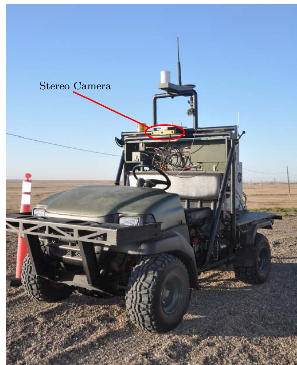
Figure 1. Experiments are performed using a large Defence Research and Development Canada (DRDC) Mule Research Vehicle (DMRV) where the sole sensor used for localization is a Point Grey Bumblebee stereo camera (highlighted in red). The experience-based speed scheduler presented in this paper is able to identify speed limits that maintain the reliability of the vision-based localization system.
