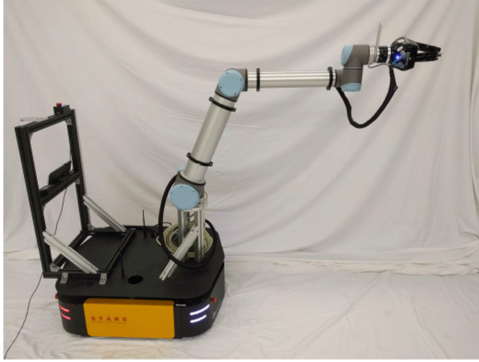
Fig. 2. The UR10 industrial manipulator used in the experiments.
