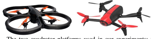
Fig. 3. The two quadrotor platforms used in our experiments; we learn a transfer learning map from the Parrot AR.Drone 2.0 (left) to the Parrot Bebop 2.0 (right).
