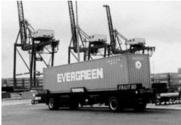
Figure 26: Photograph of completed AGV with 40 foot container load. One of the two radars can be seen at the front of the vehicle below the main deck.
